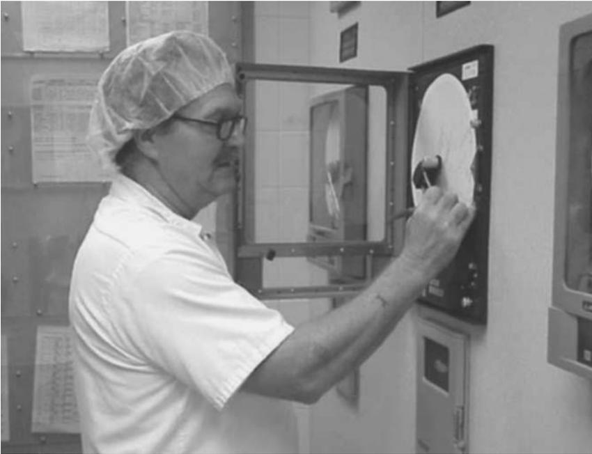
**Fig. 10.11** Operator monitoring CCP of a pasteuriser.
