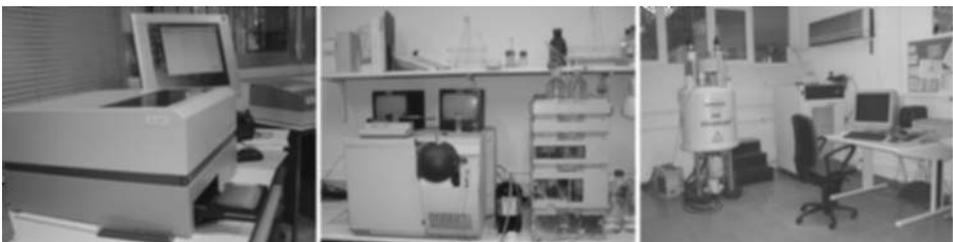
Fig. 4.3 Advanced instruments used for laboratory quality control – ELISA reader, HPLC-MS/MS and NMR spectrometer (from left to right).
